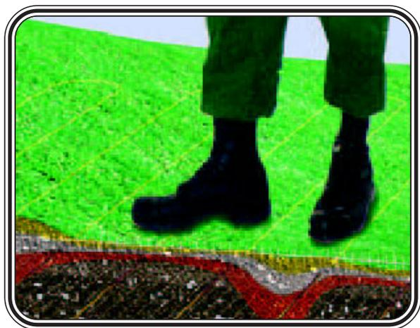
The **FiberSensor XL** buried sensor system is comprised of fiber-optic cables buried across a wide horizontal plane. The system detects pressure applied on the ground above the cable. The buried sensor cable is invisible, completely passive, and can be installed in almost any ground.
