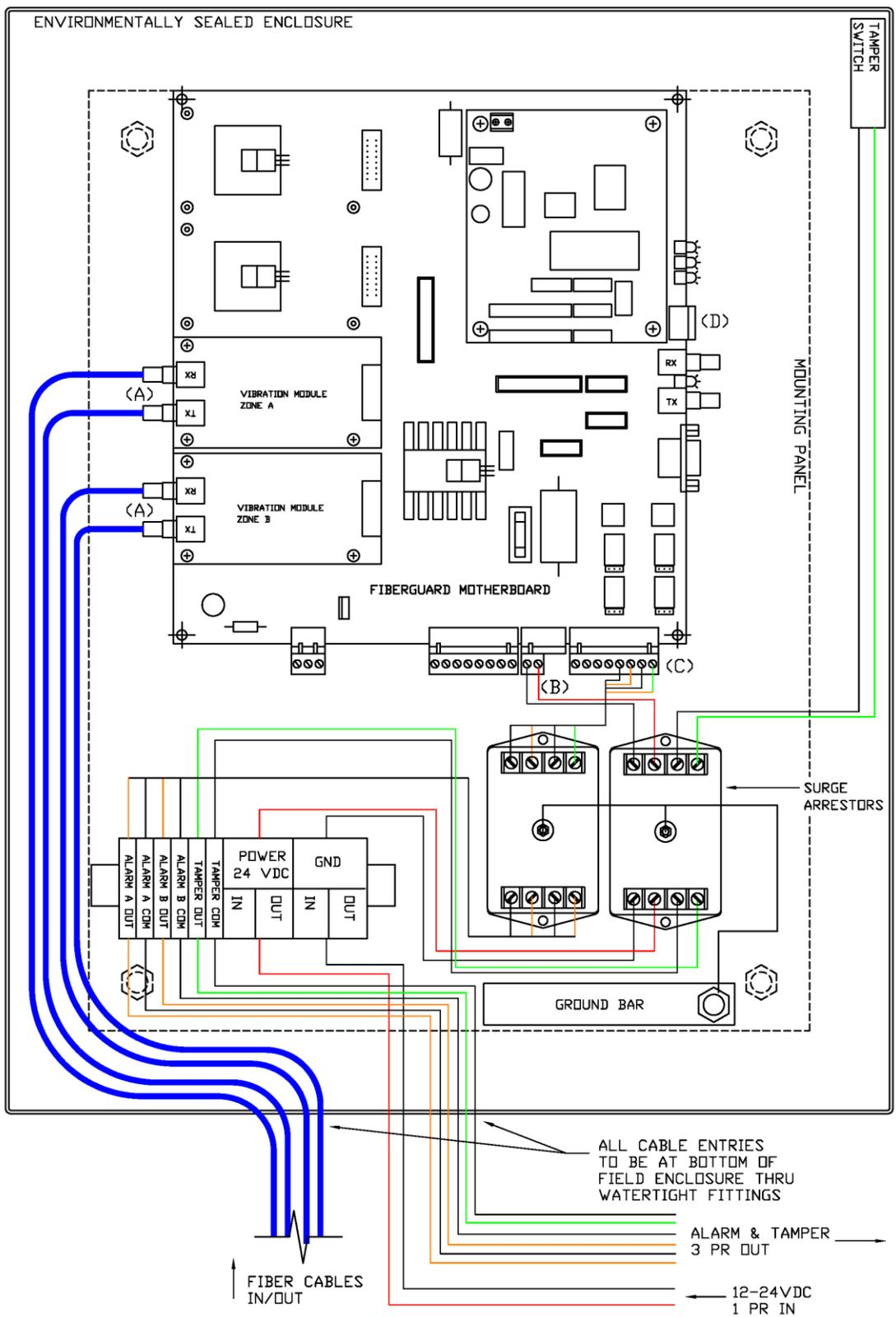
8. This example shows typical Motherboard connections in an environmentally sealed enclosure with a transponder.
