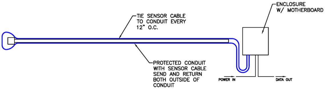
7. This example shows typical Motherboard connections in an environmentally sealed enclosure without a transponder.
