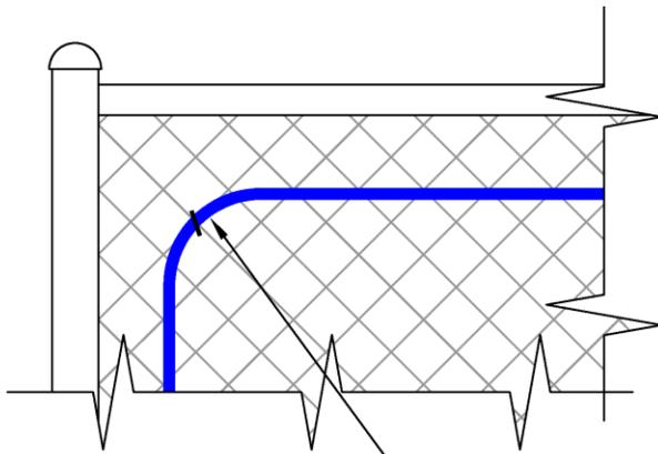
MAKE SURE WHEN ROUNDING A CORNER THAT THE TRANSITION IS SMOOTH WITH NO KINKS IN THE CABLE. SECURE WITH TIE WRAP AS SHOWN.
