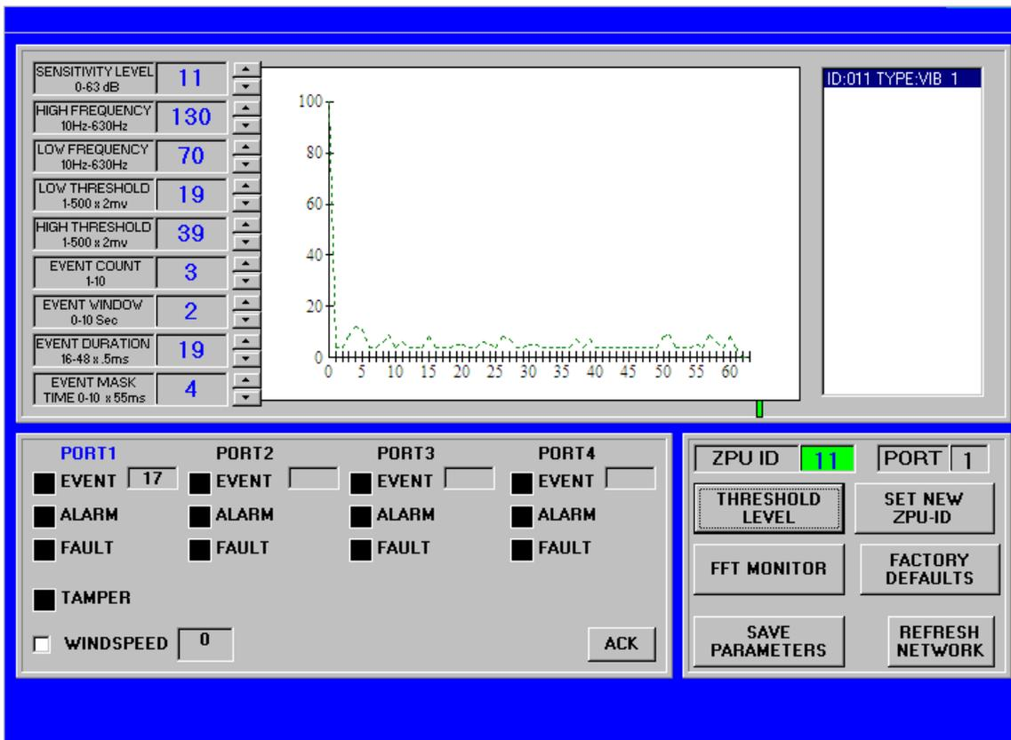
It is recommended that you let the FFT run for a short period of time while observing the FFT pattern in normal state (not in alarm condition) and setting the frequency bandwidth to exclude this value. If you observe that the response line is close to 0 then increase the sensitivity slowly but do not exceed 40 and continue to monitor. Once you exit the FFT restore the sensitivity to its previous value.
